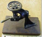
Metal label reads "Clev-Dent" or Bent Made in USA Cleveland, Ohio With a Serial No. Wheel lifts a solid plate; lever closes the gap in
